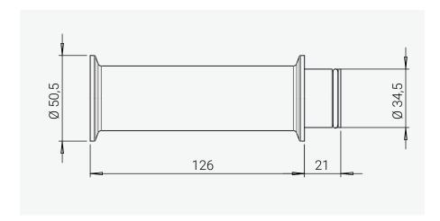
The overall diameter of the UKK is 50,5 mm.
